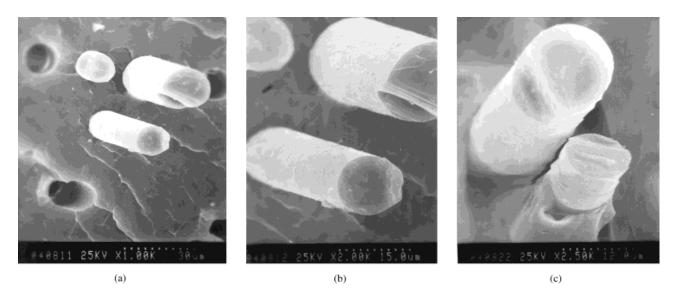
**Figure 3** SEM of impact fracture surface of (a,b)  $M_0$  and (c) tensile fracture surface of  $M_0$ .
