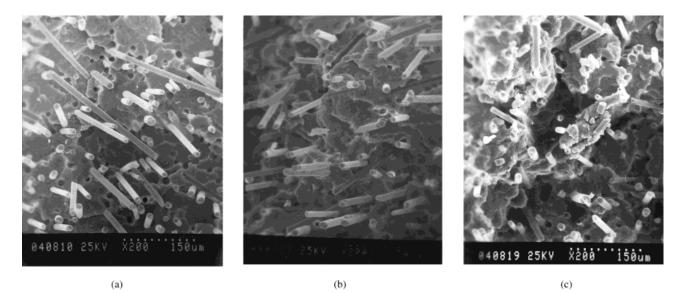
**Figure 2** SEM of impact fracture surface of (a)  $M_0$  (noncoupled GF/PP), (b)  $M_1$ , and (c)  $M_2$  (coupled GF/PP).
