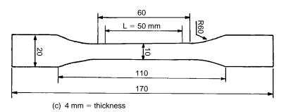
**Figure 1** Size of the test specimens: (a) for izod impact testing; (b) for flexural testing; (c) for tensile testing.
