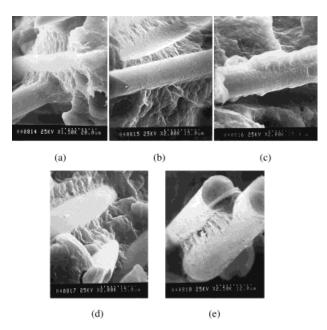
**Figure 4** SEM of impact fracture surface of  $(a-c) M_1$  and  $(d,e) M_2$ .
